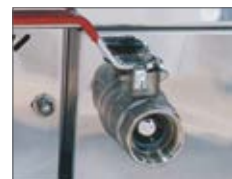
Safety lock ball valve drain
