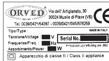
**WARNING:** It is absolutely forbidden to tamper with, engrave, alter, or remove the nameplate from the appliance. Do not cover it with adhesive tape or other such material as it must always be clearly visible.
