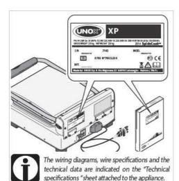
Before connecting the appliance to the mains electricity, always compare the power supply data with that of the appliance specified on the rating plate.
