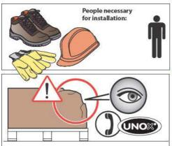
Make sure that the appliance is not in danger of tipping over during transportation. Check the package on recept for any visible damage. If damage is found, immediatly contact UNOX and DO NOT install the appliance.
