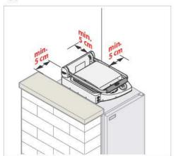
Position the appliance respecting the indicated distances in the diagram and so that the back of the oven is easily accessible for appliance connections and maintenance.
