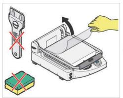
Slowly remove the protective films from the appliance: clean any glue residue with appropriate solvents without using tools, abrasive detergents or acids that could ruin the surfaces.
