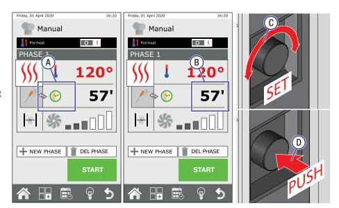
Note: For the oven to run continuously, touch the time field and turn the navigation dial to the left until the display shows INF.
