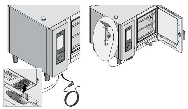
Note: When not in use, place the probe back into the magnetic support on the left side of the oven.
