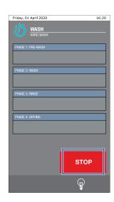
**Note:** If during a wash cycle the power to the oven is disconnected (e.g. power outage, turned off at supply) for a period less than two minutes, the oven will automatically resume the wash cycle when the power is restored.
