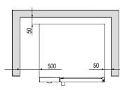
\*Clearance requirements \*Drain line must be vented
