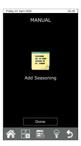
**Note:** While the message is displayed, the oven keeps running with the set temperature until "Done" is pressed (If programmed, the next phase will start).
