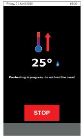
This screen displays the current temperature in the chamber (which will increase gradually) and warns that preheating is in progress. The oven requires the set temperature to be reached before introducing food into it. If necessary, the value can be changed by touching it and turning and pressing the navigation dial to the right.
