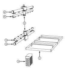
Remove scrap trays ① and wash pump inlet filter ②, where fitted, and rinse or brush clean.
