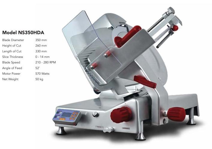
The fully automatic gravity feed belt driven slicer takes the hard work out of slicing. It is fast, clean, precise and very easy to operate and features two independent motors, one for blade rotation and the other for carriage movement.
