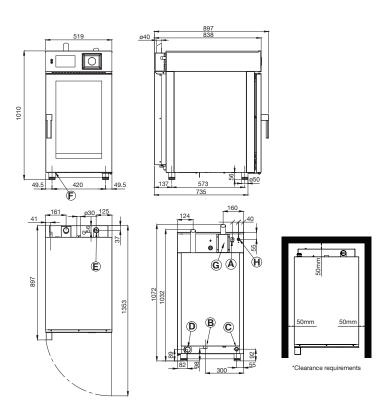
\*Heat Source: 500mm clearance from an external heat source is required in order to protect the oven control components. For of clearances under 500mm, it is mandatory for Stoddard heat sources is required under to policities with retaining a minimum clearance of 50mm to allow access to the unit. Failure to adhere to minimum clearances may void the oven warranty or add service costs due to lack of access.
