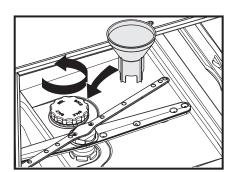
► Unscrew the salt reservoir lid and add 1.5 kg of granular (2-8 mm) regenerating salt (do not use salt tablets).
