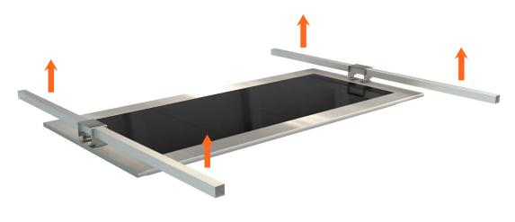
Lifting brackets are fitted to assist removing the unit from the packaging and placing in cabinetry. Use a lift bar that can fit through the 35 x 35mm square hole.( not supplied )
