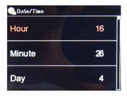
Set the new date or time, by turning knob **16** and confirm by pressing **16**.
