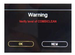
If the cartridge / tank is empty, replace it following the instructions in the following paragraph, otherwise confirm the "OK" message by pressing knob **16** to start the wash.
