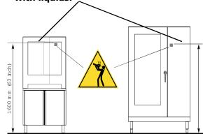
ATTENTION to avoid scalding, do not use the containers filled with liquid or food which, through cooking become fluid, at levels higher than those which can be observed.
