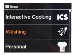
Turn knob **16**, select the wash required displayed on display **15** and confirm the start by pressing knob **16**.
