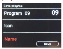
Set the name of the programme by turning the knob and confirming the selected letter by pressing knob **16.** After setting the programme name, select "OK" and confirm by pressing knob **16.**
