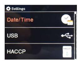
To change the date or time, highlight it by turning knob **16** and confirm by pressing knob **16**.
