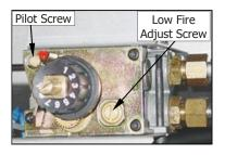
NOTE: 'Low Fire Screw' should be sealed with coloured paint on completion of low fire adjustment.
