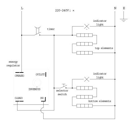
The above circuit diagram has been provided to assist qualified technicians, Only Birko Foodservice agents or Recommended Qualified Technicians should carry out repairs if needed. Do not remove any components or service panels on this product.
